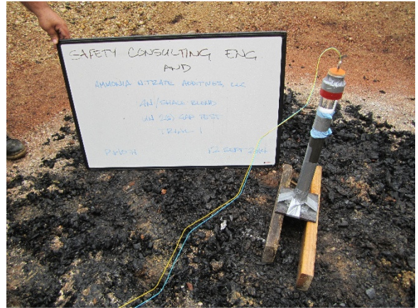
Figure 4. UN 2(a) Gap test, pre-test
