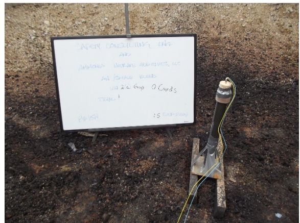
Figure 2. UN 1(a) Gap Test, pre-test
