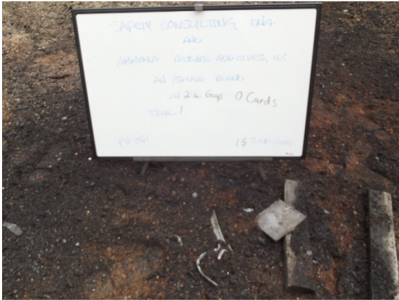
Figure 3. UN 1(a) Gap test, post-test
